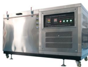
Figure 30 – Example cold chamber
