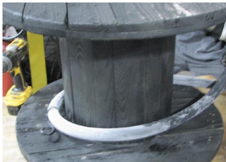
Figure 31 – Example tool for performing bend test (reel or mandrel)
