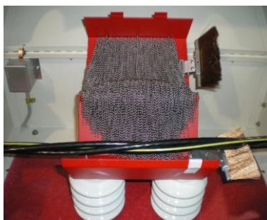
Figure 43 – Spark tester (open)
