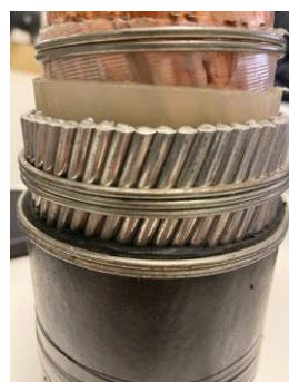
Figure 12 – Galvanized steel armour
