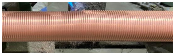
Figure 2 – Longitudinally applied and corrugated copper tape
