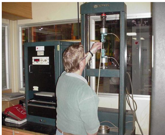
Figure 18 – Universal testing machine used for tensile and elongation testing
